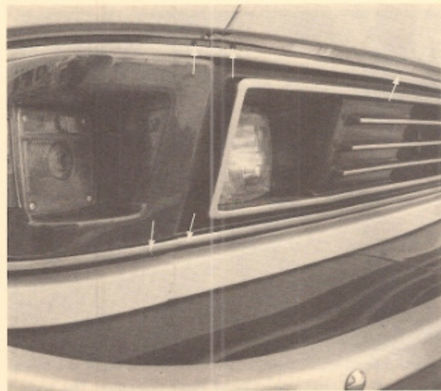
Figure 69 — Grille Removal: Remove 13 No. 6 pan head Phillips, black-painted heads. Screw locations include 3 at each end, 3 at the center, and 4 across the top.
