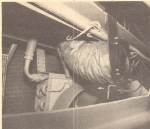
Figure 72 – Air Inlet Hose Removal: Remove the 4 1/2"-diameter air inlet hose that is fastened to the back side of the firewall. With the inlet hose disconnected, you can begin removal of the upper air deflector. Starting with the 1981 models, the hose can be disconnected at the grille.
