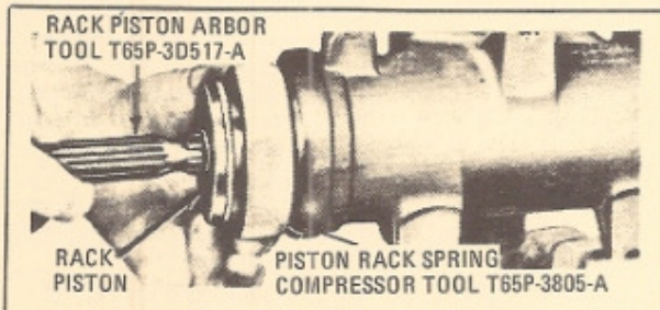
Figure 147 — Installing Rack Piston
